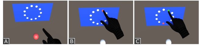
Figure 3: Reaching Task : (A) 3D Sphere is highlighted red, indicating the start of the interaction. (B) After the initial selection, the user moves to select the highlighted red target in the 2D plane. (C) After selecting that, the target colour changes to green and a new target is highlighted in red. The user then drags to that.
