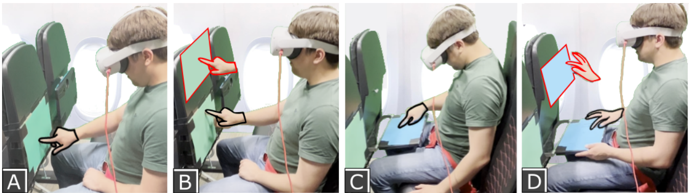
Figure 1: Using passive haptics surfaces in planes for interaction. (A) shows how the seat-back in front can be used as a passive haptic surface; (B) using translation remapping to create a more comfortable experience; (C) shows the use of a horizontal tray table for passive haptic input; and (D) using translational and rotational remapping for a more comfortable interaction.
