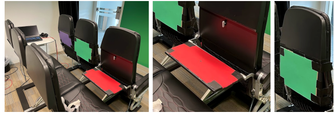
Figure 2: From Left to Right: Plane Seats and the surfaces used in the experiment; Horizontal Tray table (Red); Vertical Surface (Green) (the purple surface was not used in this study).
