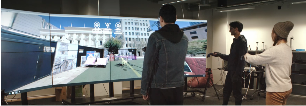
Figure 1: Users collaborating using the TeleGate system. A shared immersive display is used to prevent crucial facial and bodily cues from being obscured by VR headsets. Virtual objects are realistically blended into live or pre-recorded 360° video using real-time lighting estimation, allowing this display to act as a “window” into remote spaces that can be manipulated using handheld controllers.
