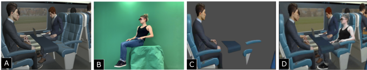
Fig. 1. Using the Oculus Mixed Reality Capture Tool, the composition of A (background), B (chromakey reality) and C (foreground) gives the final result D - where real video is composited in a way that respects the depth of the virtual imagery. In this way, we can create video clips that demonstrate an interaction technique in a specific context with high fidelity.
