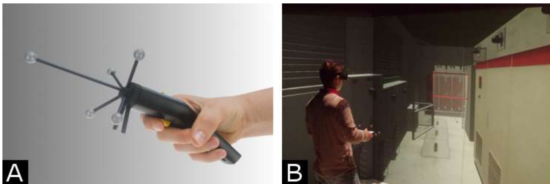
Figure 2.14: Devices used to control virtual techniques : (A) Flystick (B) Tablet with 6DoF Tracking
