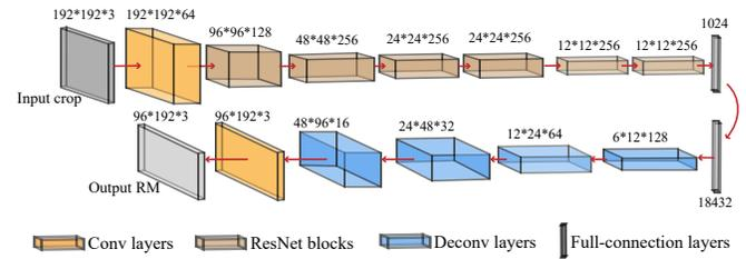
Fig. 3: Overview of a single CNN architecture.
