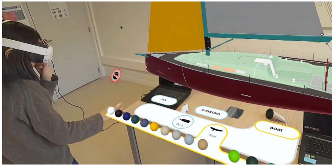
Fig. 3: Couple Interaction in Shared VR Environment: From the first user's perspective, the second user configures the color of the virtual sailboat via the shared user interface, which is rendered simultaneously.
